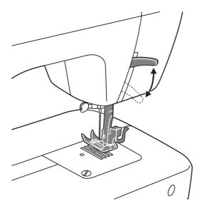
When sewing several layers or thick fabrics, the presser foot can be raised a second stage for easy positioning of the work.
