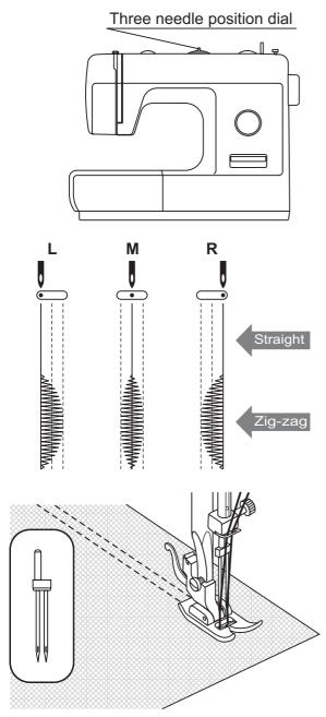
The needle position can be altered with the "Three needle position dial". For normal work, the needle position is middle. For edge stitching or sewing parallel lines of top stitch, select needle position left or right.
