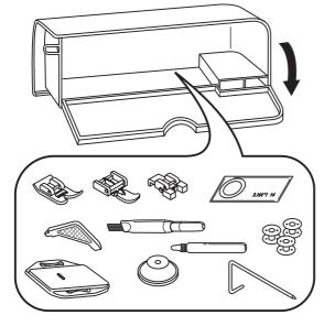
Keep the snap-in sewing table horizontal, and push it in the direction of the arrow.
